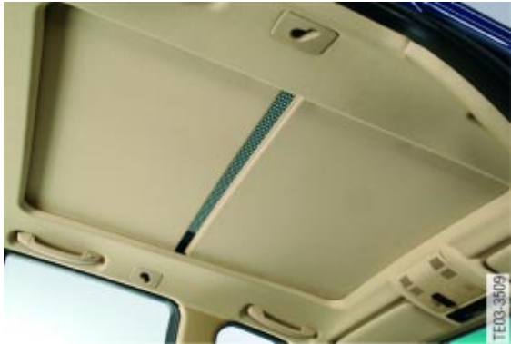
Ventilation Gap E61
